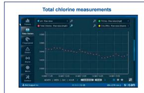
When drinking water is disinfected through chlorination it is necessary to continuously control the actual chlorine level. This figure shows the total chlorine measurements of one of the monitoring stations in Alberta.
